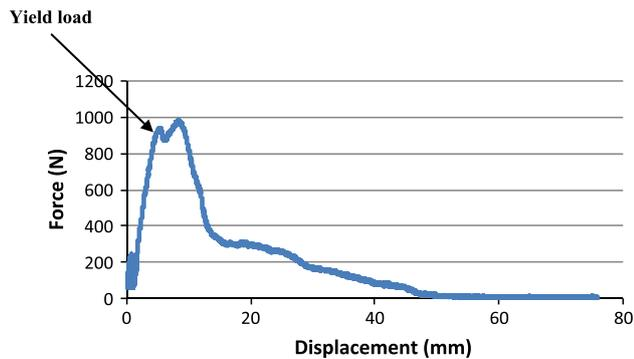
**Fig. 4** Single-cycle load-to-failure test. The yield load corresponds to the inflection point of the curve. The slope of the quasi-linear curve represents the stiffness (N/mm) of the fixation–tendon construct
