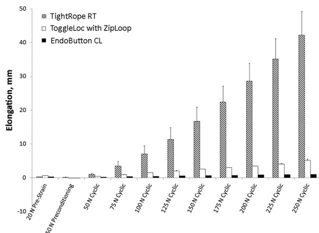
**Figure 3.** The average loop extension (in millimeters) after 500 cycles at each 25-N load increment for all devices (without suture knotting).
