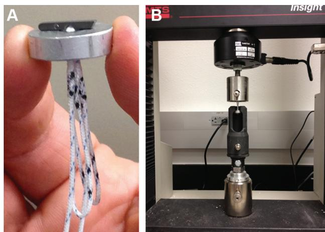
**Figure 2.** (A) Device mounted onto the stainless steel plate. (B) The test setup showing the mounting of the fixation device and the stainless steel plate and rod used to conduct the test.
