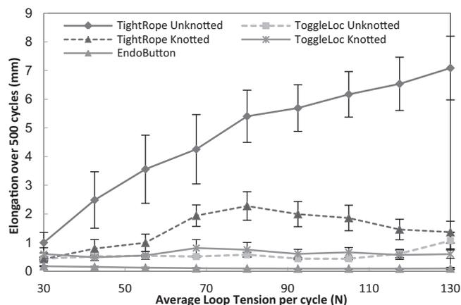
**Figure 4.** Relative extension over each block of 500 cycles for the 3 grafts (with or without suture knotting). The unknotted TightRope shows a trend of increasing elongation with increasing load, while the EndoButton shows no increase in elongation with load and a decrease in relative extension with an increasing cumulative cycle number. No statistical difference with knotting is observed for the ToggleLoc.
